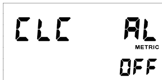
Figure 41a PROGRAMMING MODE (Clock Alarm - On/OFF)
