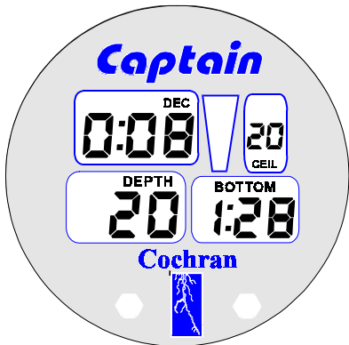
FIG-7 EMERGENCY DECOMPRESSION MODE DISPLAY
